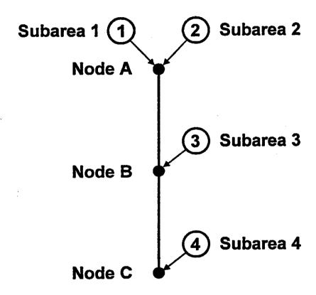
Figure 2. Model Schematic for Four Subareas and Two Hydrograph Routing Links.
